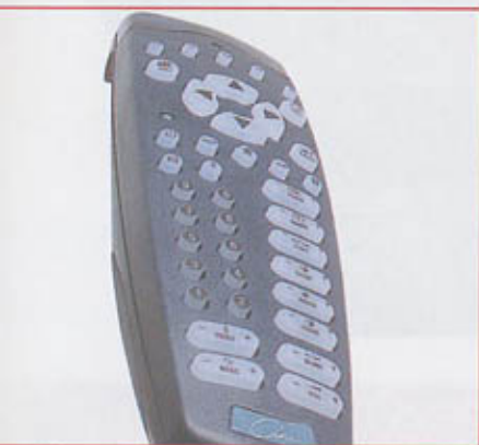
The remote is backlit for use in the dark
